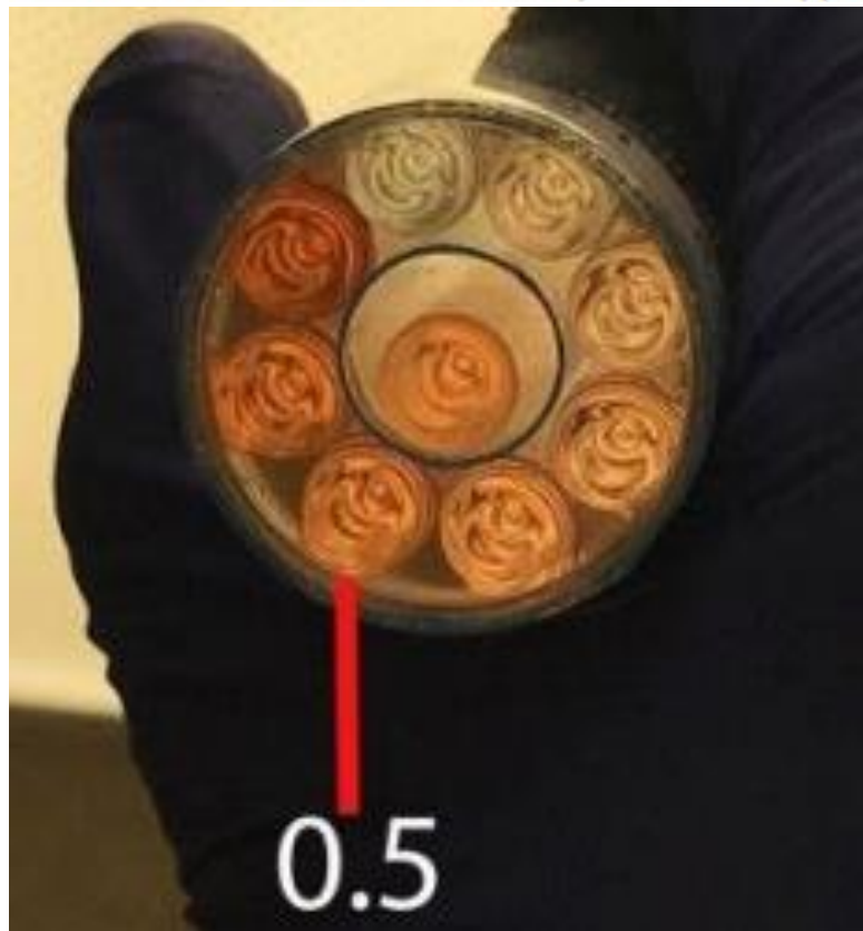
Picture 1: CHEMetrics® Color Comparator at 0.5 ppm
